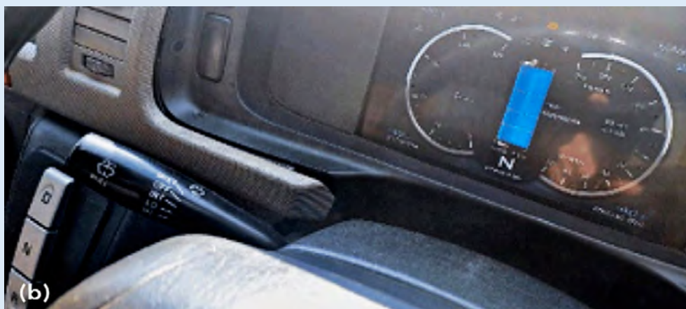
FIGURE 19. The electric retrofitted minibus taxi (original model from 2009) (a) Completed retrofitted taxi. (b) Retrofitted electric vehicle's electronic dashboard and controls (Drive (D), Neutral (N), Reverse (R)) (Lacock, et al. , 2023)
